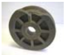
WORN CABLE ROLLER
